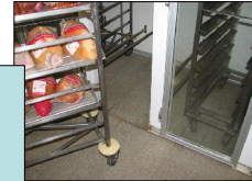
Upright fridge cabinets (and bakers' ovens) with continuous level floor surface allows stock to remain on trolleys and reduces resistance when pushing/ pulling
