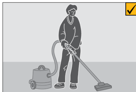
Worker is able to complete task in an upright position as wand length can be adjusted to worker's height.
