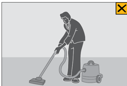
Vacuum cleaner wand length is short resulting in awkward posture.
