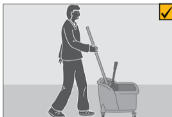
Bucket with wheels removes need to bend and lift.
