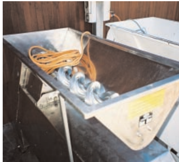
Example of an unsafe unguarded crusher de-stemmer at a Margaret River winery.
