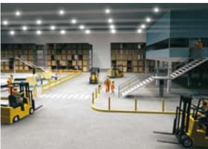
Mobile plant operated in areas where people work may cause injury through collision. Traffic control and segregation are forms of control.
