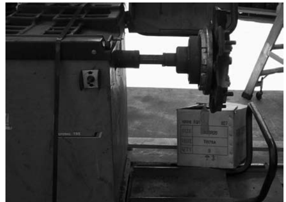
Hydraulic tyre lifter retrofitted to a wheel balancer
