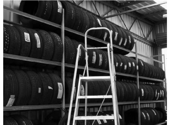
High racking system with platform ladder
