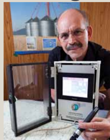
Henk de Graaf with the Aeration Control, a new innovation to automate the process of drying, cooling and maintaining grain to reduce energy consumption.
